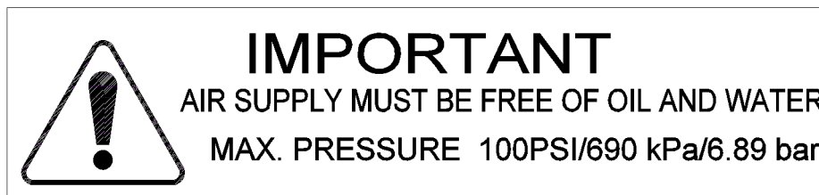
Figure 1.1 Caution label on the 2000X aed Actuator for the factory air supply
